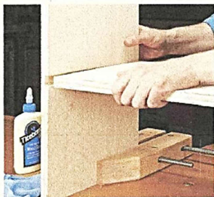
▲ A handscrew provides support to hold cabinet sides upright while putting together a complicated assembly.
