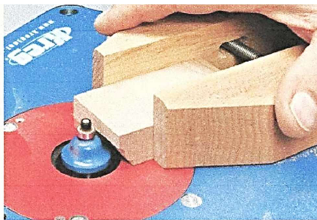
▲ Handscrews are great for machining small parts, thanks to the wood jaws.
