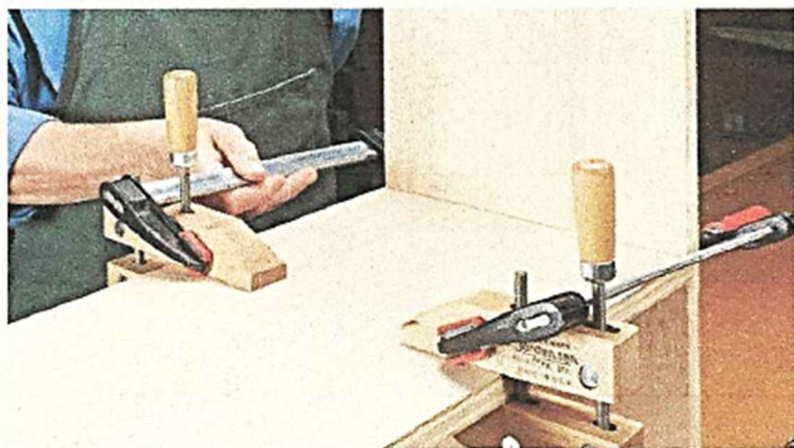
▲ For a wide assembly where your clamps don't have enough reach, attach handscrews to the dividers. Then clamp across the sides and the handscrews to draw the assembly together.
