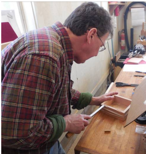
Rich creates the mortises for the really nice hinges
