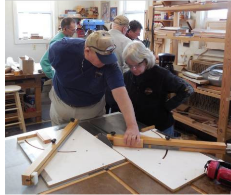
Andy shows Vicki the proper technique for using the Dubby Board to cut the 45 degree sides
