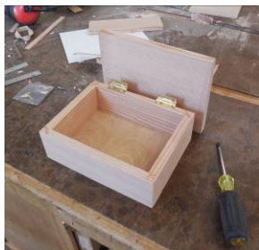
Box with hinges - notice the lid is still one piece
