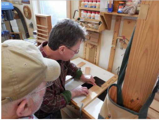
Rich routes the grooves for the bottom after getting guidance from Don
