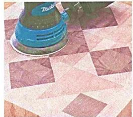
▲ Tough end grain requires a coarse disc to remove the score marks. Then step up to higher grits for a glass-smooth surface.
