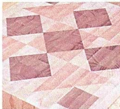
▲ The router work is complete when the surface has a uniform look with faint score marks left from the bit.
