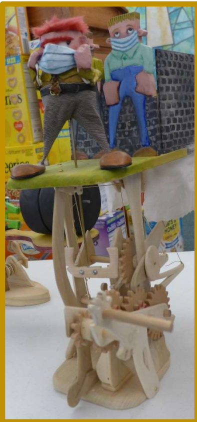
Covid theme automation, showing the mechanism. Don saves time by 3D printing his gears in wood resin.
