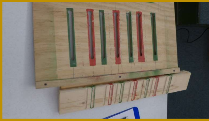
Rodger Young made this display box for Japanese tea cups. He also showed us the jigs he used to make the router cuts required.
