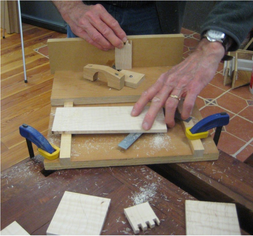
Router jig for making finger joints.
