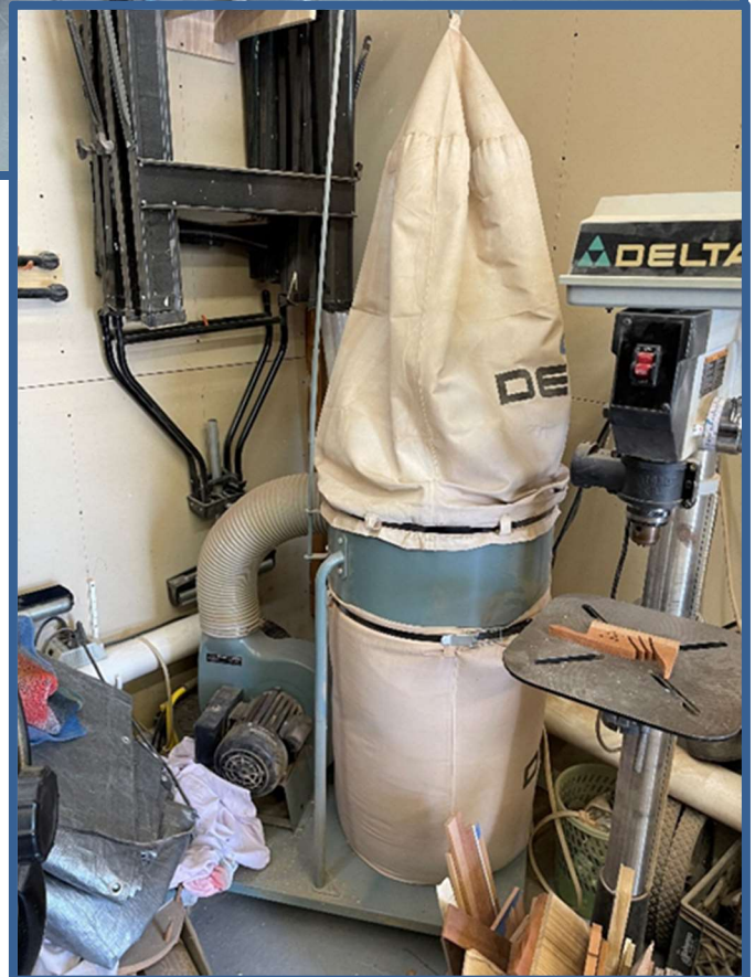
Three HP dust collector in the back corner pulls in the dust from multiple locations throughout this side of the shop as well as the center where the tablesaw and bandsaw reside.
