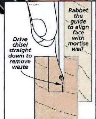
▲ A simple guide block helps you keep the paring cuts square.
