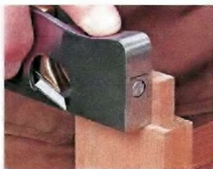
▲ A shoulder plane makes quick work of removing saw marks on cheeks and stepped shoulders.
