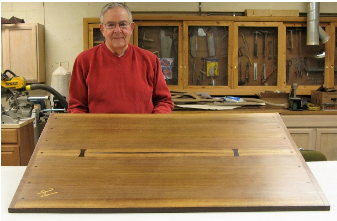
Karl Hoke shows his quarter-sawn walnut table top with natural edges, butterflies, and square pegs holding rose wood breadboard ends. Finish is polyurethane.
