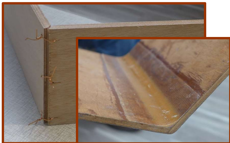
Boat seams stitched (left) and glued (right)
