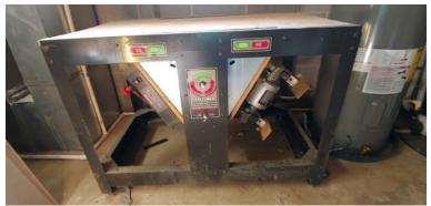
The second tool is a Craftsman miter chop saw that is mounted on a movable work surface with extensions.
